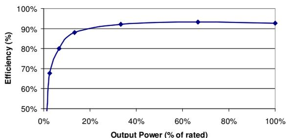
Graph 1: Typical dependency of the conversion efficiency on the output power
