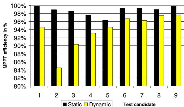
Graph 8: Comparison of average weighted static and dynamic MPPT efficiencies for the different test candidates
