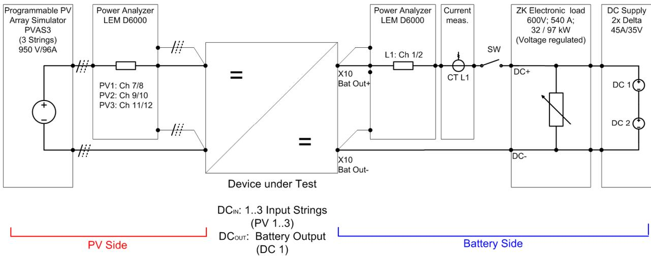
Graph 4 : Test setup for MPPT charge controllers at AIT<sup>4</sup>
